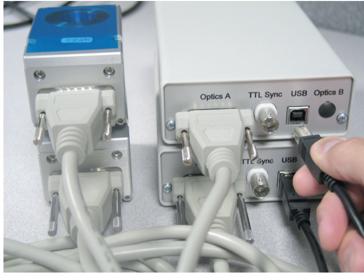
Figure 8. 26-pin HD D-Sub cables connect to the VariSpec optics modules and electronics controller modules; USB cables connect to the electronics module and computer
